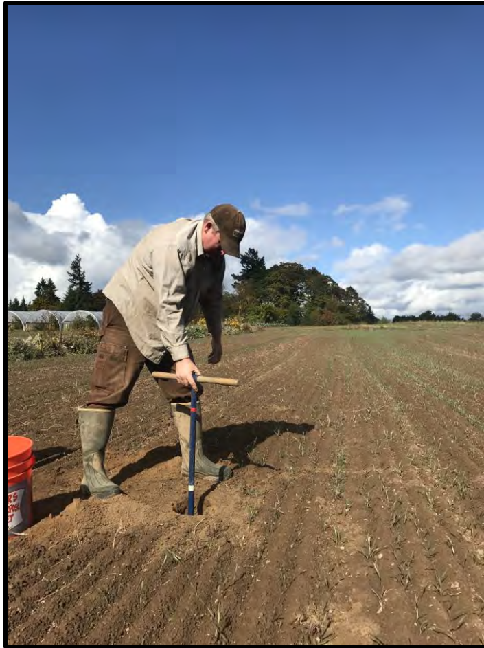
Figure 4: Soil Sampling to a depth of 24" depth newly seeded winter cover crop, October 2017
